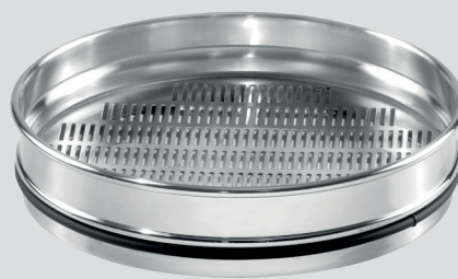
Grain sieve made in accordance with ISO 5223
